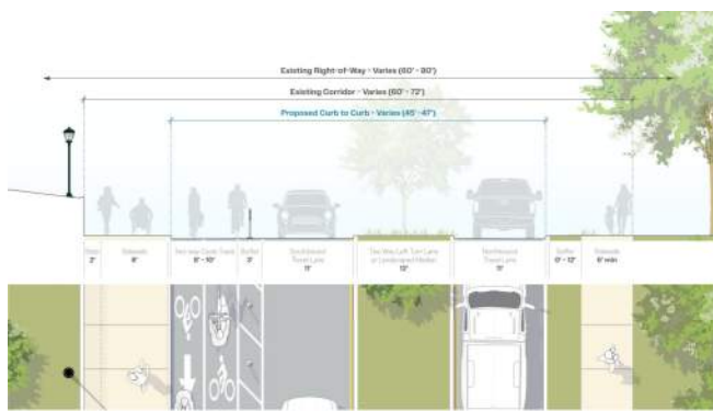
Alternative 2: Sidewalk with Two-way Cycle Track (A-A) Clarkston Safety Action Plan | North Indian Creek Drive | Typical Sections
