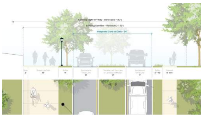
Alternative 1: 13' Shared Use Path with Landscape Buffer (A-A) Clarkston Safety Action Plan | North Indian Creek Drive | Typical Sections
